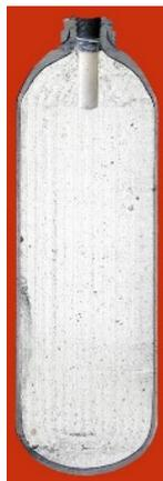
To further protect the cylinder from a flashback, a flashback/flame arrestor shall always be used with acetylene cylinders. If flashback does reach the cylinder, the porous material would normally quench this decomposition reaction. See EIGA Safety Info 05, *Flashback and flashback arrestors* [1]
